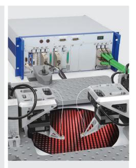
F-712: FAB-proven, ultrafast Nand NxM-axis alignment for multiple interacting couplings (as in multi-channel SiP devices). Real-time simultaneous optimization and tracking is built in. Integrated coarse/fine control; 2 nm resolution.
