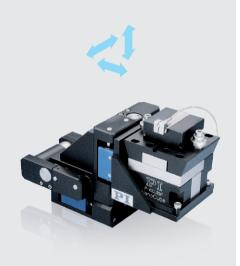
F-131: Modular, compact coarse/ fine XYZ alignment stack. Highspeed, piezo-based scanning and alignment algorithms. Control via F-712 with integrated firmware real-time alignment algorithms, or via modular PI controllers with software alignment modules.
