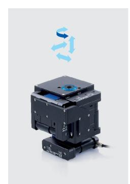
F-131: 3 linear axes, 50 nm step size, to 25 mm travel per axis, plus 1 rotary axis optional.
