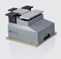
H-206: 6-DOF, 0.1  $\mu$ m / 0.1 mdeg resolution, built-in alignment algorithms. One- or two-sided alignment. Long travel (up to 15 mm / 13 degrees).
